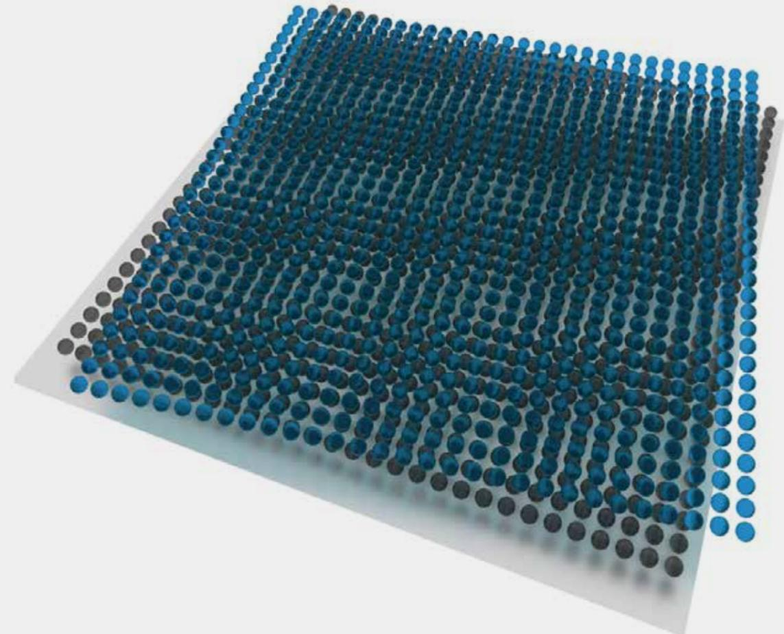
A model of a moiré pattern. When two 2D crystals (black and blue) are superposed, interference patterns occur, in turn changing the physical properties of the whole assembly.
