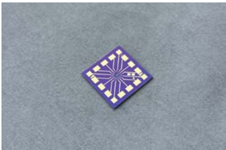
One of the devices made by the researchers (1cm by 1cm in size). A nanowire network sits in the centre (too small to see) and is overlaid by a film of memristive molecules. Gold electrodes extend outwards to contact pads around the edges and these can connect to external measurement devices. The base is a silicon wafer with an insulating silicon dioxide layer on top.
