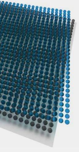
A model of a moiré pattern. When two 2D crystals (black and blue) are superposed, interference patterns occur, in turn changing the physical properties of the whole assembly.
