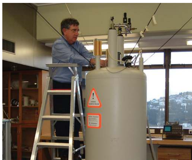
Paul Callaghan loading a sample into the superconducting magnet
